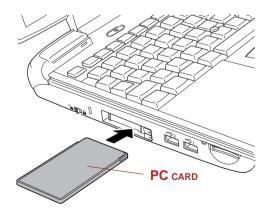
Figure 8-1 Inserting the PC card
